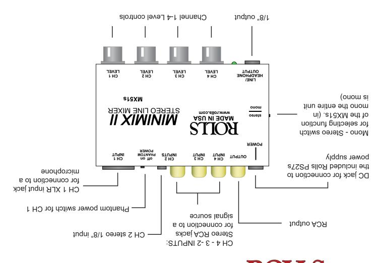
The MX51s is a four channel mixer designed for Audio and Visual applications. Channel 1 has a microphone XLR input with selectable phantom power. Channel 2 has both 1/8" and RCA inputs. Channels 3 and 4 have RCA inputs. The MX51s also features a 1/8" line or headphone output that will drive up to 600  $\Omega$ headphones. It has enough output level to connect to any power amplifier. The MX51s is powered by an included ROLLS PS27s adapter.
